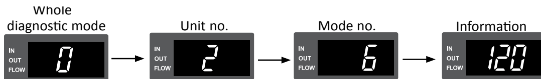
Figure 40. This example shows the steps for displaying the outlet temperature for unit 2 in a linked system.
